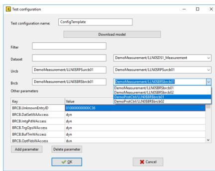
Editable configuration files. DUT data model can be imported and used for test configuration.
